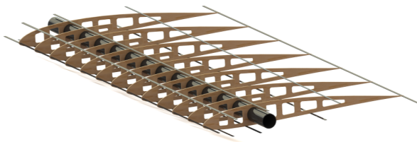
Fig. 6: This figure is a wing structure model developed for the prototype solar UAV. High modulus pultruded carbon fiber stringers are located at the perimeter of the wing to increase bending rigidity and maintain the airfoil cross section between the ribs. The center spar is a filament wound carbon fiber tube which provides torsional rigidity and is the primary structural component of the wing.
