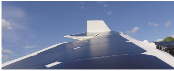
Fig. 18: In-flight side view of the SUAV:Q showing the control surface actuation resulting in a change in solar irradiance on the control surface.
