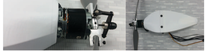
Fig. 10: Closeup of variable pitch linkage with a custom aluminum clevis and side view of a propulsion system unit and wind tunnel testing mount.
