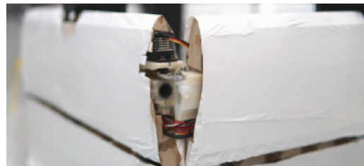
Fig. 8: Fabricated hinge installed into the transforming airframe and driven into the quad-rotor position.
