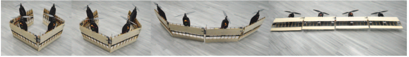
Fig. 5: Ground transformation from quad-rotor to fixed-wing states using the transformable airframe.
