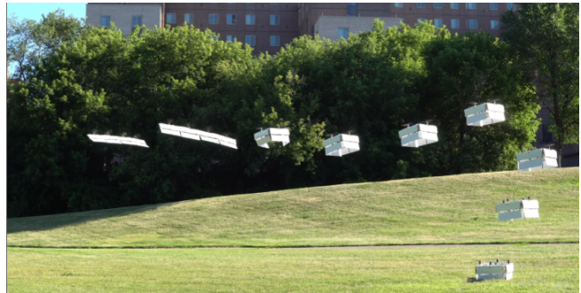
Fig. 1: MIST-UAV Prototype performing multi-rotor to fixed-wing transformation.
